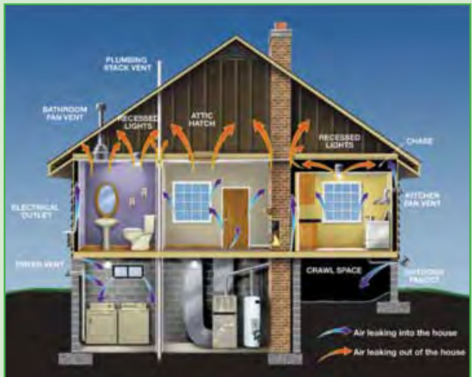
Stopping air leakage into and out of a home is important for energy savings and protection from the damaging effects of moisture. www.EnergyStar.gov
